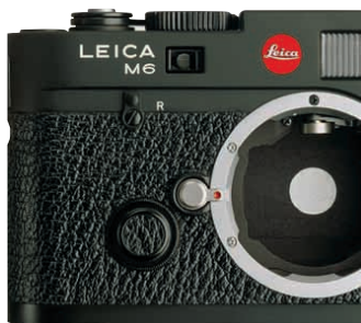
Reflects light onto the silicon photo diode in the upper interior of the camera for accurate exposure determination: the white spot on the shutter curtain.
